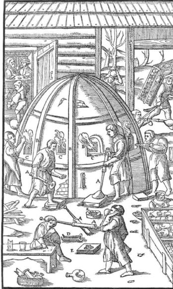
A. PIPAS DE SOPLO B. RESQUICIOS C. EMBOCADURAS DE MÁRMOL
